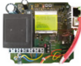
NDA008 Repeater module with integrated router.
